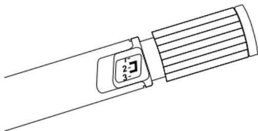
5. Hold the InPen system so that the needle is pointing up and tap the cartridge to collect any air at the top.
