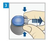
Remove the disconnect cover by gently squeezing the sides and pulling it away from the insertion device.
