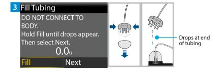
Remove the white cap from the site connector by squeezing the sides of the site connector then pulling the white cap off. Select **Fill** and keep holding
