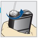
Remove the used reservoir from the pump.
