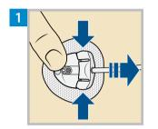
To disconnect, gently hold the cannula housing steady with your finger. Then squeeze the sides of the site connector and pull it out from the cannula housing.
