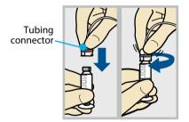
Gently push the tubing connector onto the reservoir. Turn the connector clockwise until it is locked into place.
