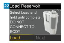
Select **Load** and hold @until the check mark appears on the screen. **Do not** connect the infusion set to the body.
