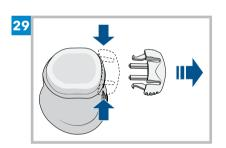
Remove the disconnect cover from the insertion device by gently squeezing the sides of the disconnect cover then pulling it away from the insertion device. Keep the disconnect cover for later use.
