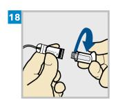
Twist the plunger counter-clockwise to loosen it and to remove it.
