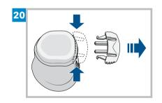
Remove the disconnect cover from the insertion device by gently squeezing the sides of the disconnect cover then pulling it away from the insertion device. Keep the disconnect cover for later use.
