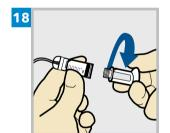
Twist the plunger counter-clockwise to loosen it and to remove it.
