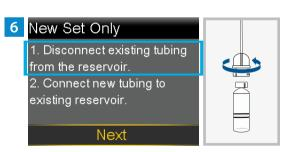
Disconnect the tubing connector of the used infusion set tubing from the reservoir. Place the reservoir on a clean surface. Do not throw the reservoir away.
