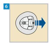
Remove the disconnect cover by squeezing the sides and pulling away from the cannula housing.
