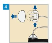
Remove the white cap from the site connector by squeezing the side of the site connector then pulling the white cap off.
