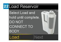
Select **Load** and hold ountil the check mark appears on the screen. **Do not** connect the infusion set to the body.
