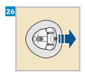
Remove the disconnect cover by squeezing the sides and pulling away from the cannula housing.
