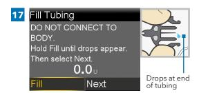
Select **Fill** and keep holding **O** until there are no air bubbles visible in the tubing, and there are drops at the end of the tubing.
