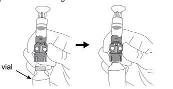
4. Push down on the plunger to pressurize the vial.
