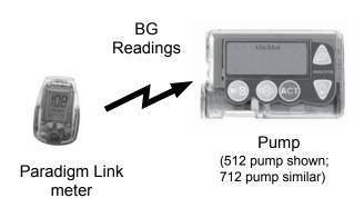
When the pump is idle (at the HOME screen), it will beep or vibrate when it receives a BG reading from the Paradigm Link meter. The reading will appear on the pump screen.
