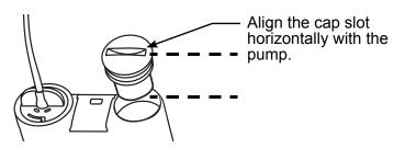
5. Turn the battery cap clockwise 4 half-turns so the slot is aligned horizontally with the pump as shown here:
