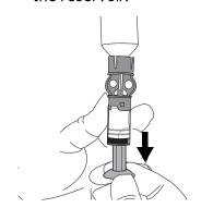
6. Tap the side of the reservoir to make any air bubbles rise to the top of the reservoir.
