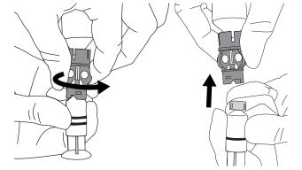
**9.** Put the tubing connector on the reservoir. Turn it clockwise to secure.
