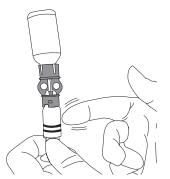
7. Slowly push up on the plunger just enough to remove any air bubbles from the reservoir.
