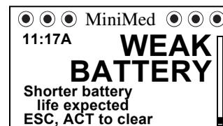
Always make sure to install a NEW battery in the pump.
