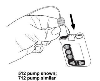
3. Turn the tubing connector approximately 1/2-turn clockwise until the connector is seated. The tubing connector should be aligned horizontally with the pump case as shown here.
