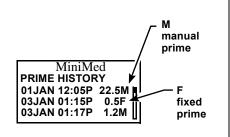
4. Scroll through the list of prime deliveries. The "F" at the end of the text line indicates a fixed prime. An "M" indicates a manual prime. Exit the menus.
