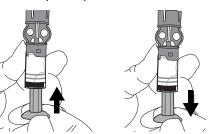
8. While holding the reservoir, turn the transfer guard counter-clockwise then pull straight up to remove it from the reservoir.
