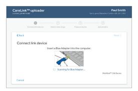
Insert the blue adapter into the USB port on the computer.
