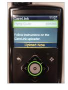
Pair the pump. At the pump home screen, press and hold the down arrow key until CareLink™ menu appears. Enter the pump code displayed on pump into CareLink™ Uploader. Select Next
