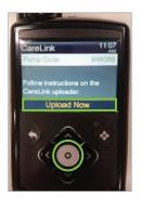
On the pump select **Upload Now**. This step must be completed for data to begin the upload process. Screen timeout on the pump will occur if **Upload Now** is not pressed within 2 minutes after accessing the menu.
