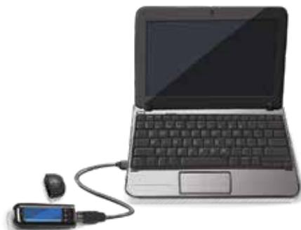
4. When charging is complete, the test strip port light will turn off. You can then unplug your meter. For more information on using your meter, see the User Guide found in the meter box.
