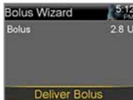
NOTE: Active Ins. adjust. is the active insulin from previous boluses that is adjusted (subtracted) from the correction dose. In this example, there was no active insulin to subtract.
