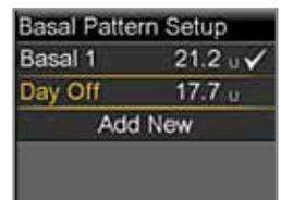
NOTE: The Basal pattern that your pump is currently using has a check mark next to it.
