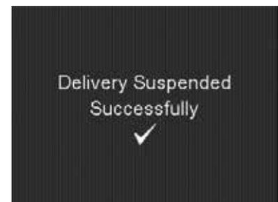
Notice that the Home screen has changed. The pump will beep and/or vibrate every 15 minutes while the pump is manually suspended.
