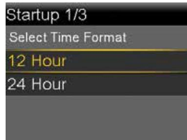
Select **12 Hour** (AM/PM) or press **v** to **24 Hour** and press **o**. *This example uses 12 Hour.*
