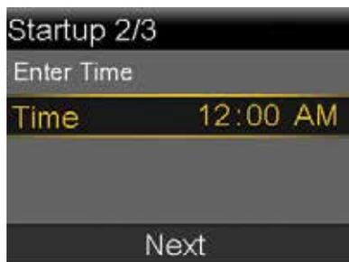
The hour will be flashing. Press **^** / **v** to the correct hour and press **o**.
