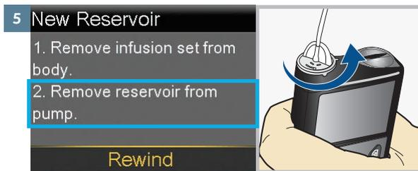
Remove the used reservoir from the pump.
