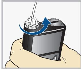
Remove the used reservoir from the pump.
