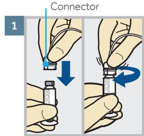
Gently push the tubing connector onto the reservoir. Turn the connector clockwise until locked. You will hear a click.
