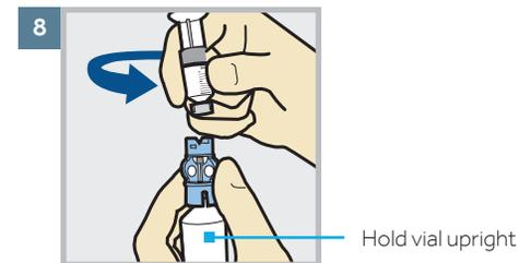
To avoid getting insulin on the top of the reservoir, turn vial over so it is upright. Hold transfer guard and turn reservoir counter-clockwise and remove from transfer guard.
