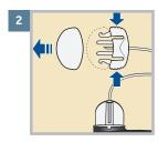
Remove the white cap from the site connector by squeezing the sides of the site connector then pulling the white cap off.
