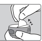
3. Squeeze the three raised markings on both sides of the mio lid. Lift and remove the lid.
