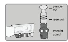
2. Pull the plunger down to fill the reservoir with air.
